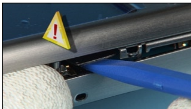
14. Carefully unlock this flex foil connector.
